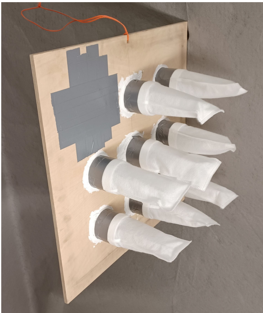
Picture 1. Filter installation in adapting panel allowing eight filter units parallel testing. Any possible leakages around the filter were duct taped.
