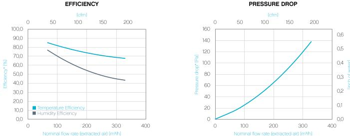
\*Based on a CORE height of 500 mm, test conditions following DIN EN 3081997-06 (intake air. temp. 5 °C, humidity 70 %; extracted air. 25 °C, humidity 50 %)
