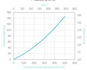
\*Based on a CORE height of 500 mm, test conditions following DIN EN 3081997-06 (temp. intake air: 5°C; temp. extracted air: 25°C)
