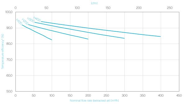
\*Test conditions following DIN EN 308:1997-06 (temp. intake air: 5 °C; temp. extracted air: 25 °C)
